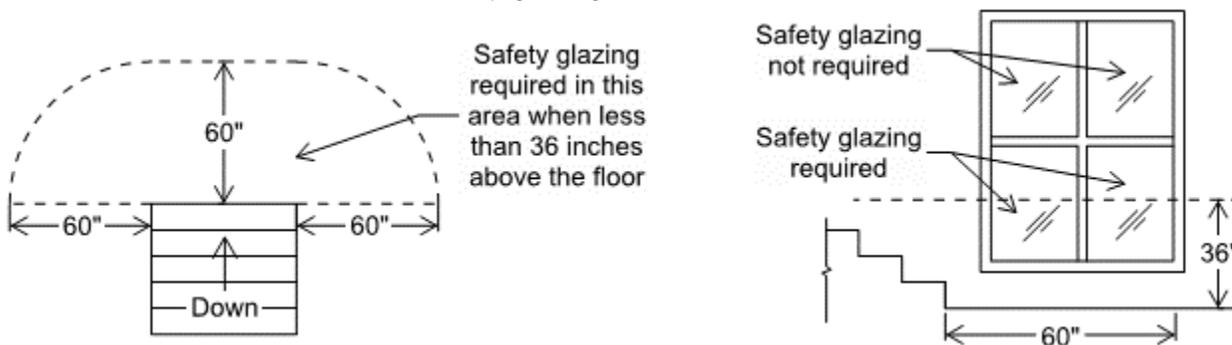
**7. Glazing Adjacent to Stairs and Ramps:** Glazing where the bottom edge is less than 36 inches above the plane of the adjacent walking surface of stairways, ramps, and landings between stair flights and ramp runs, must be safety glazing.
