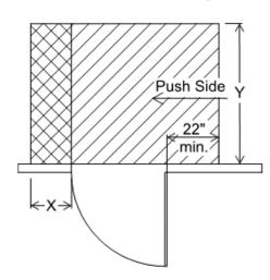
Y = 48" min. and X = 12" min. if door has a latch and a closer.
