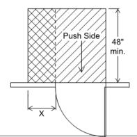
X =12" min. if the door has both a closer and a latch.
