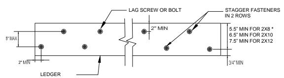
\*DISTANCE CAN BE REDUCED TO 4.5" IF LAG SCREWS ARE USED OR IF BOLT SPACING IS REDUCED TO THAT OF LAG SCREWS TO ATTACH 2X8 LEDGERS TO 2X8 BAND JOISTS.
