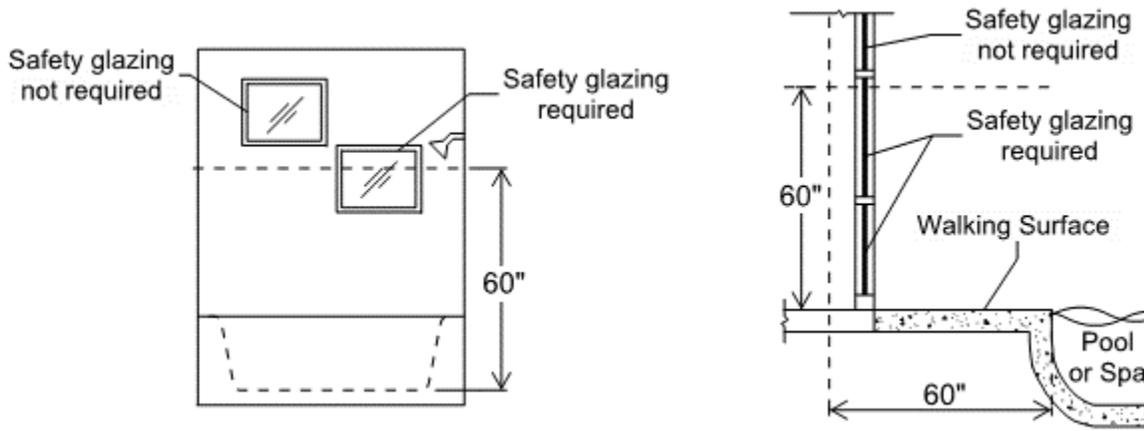
**6. Glazing Adjacent to Bottom Stair Landings:** Glazing adjacent to the landing at the bottom of a stairway where the glazing is less than 36 inches above the landing and within a 60 inch horizontal arc from the bottom tread must be safety glazing.
