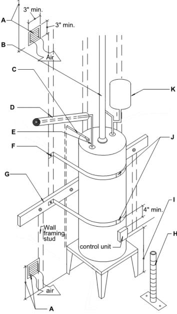
**Note:** R-10 insulation required under electric water heaters installed on concrete floors or in unconditioned space.
